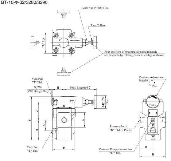
★ There are two threaded connection pressure ports. They can be connected each other in-line; one as inlet and the other as an outlet or the valve can be used by plugging one of the pressure ports.
